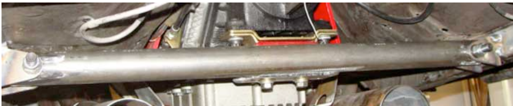
The fabricated transmission cross member.
