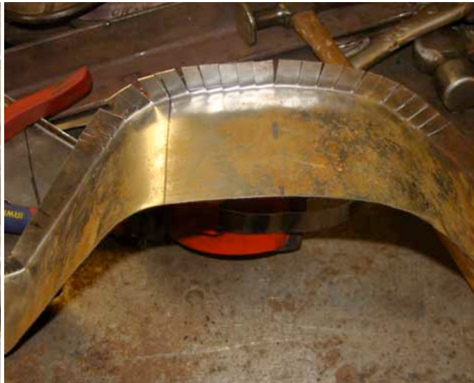
I cut slots into the flange to allow bending without a fancy machine. Not that I wouldn't like to have a fancy machine!
