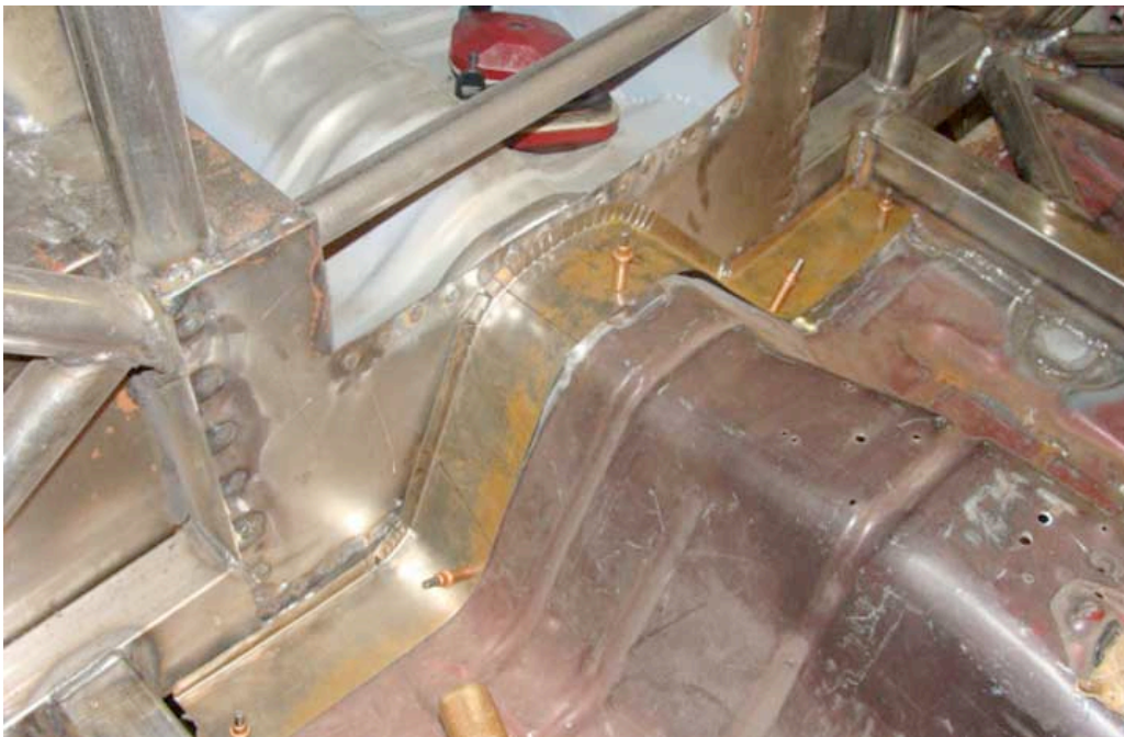
Here is the tunnel piece temporarily held in place by Clecos. I later spot welded it into position.
