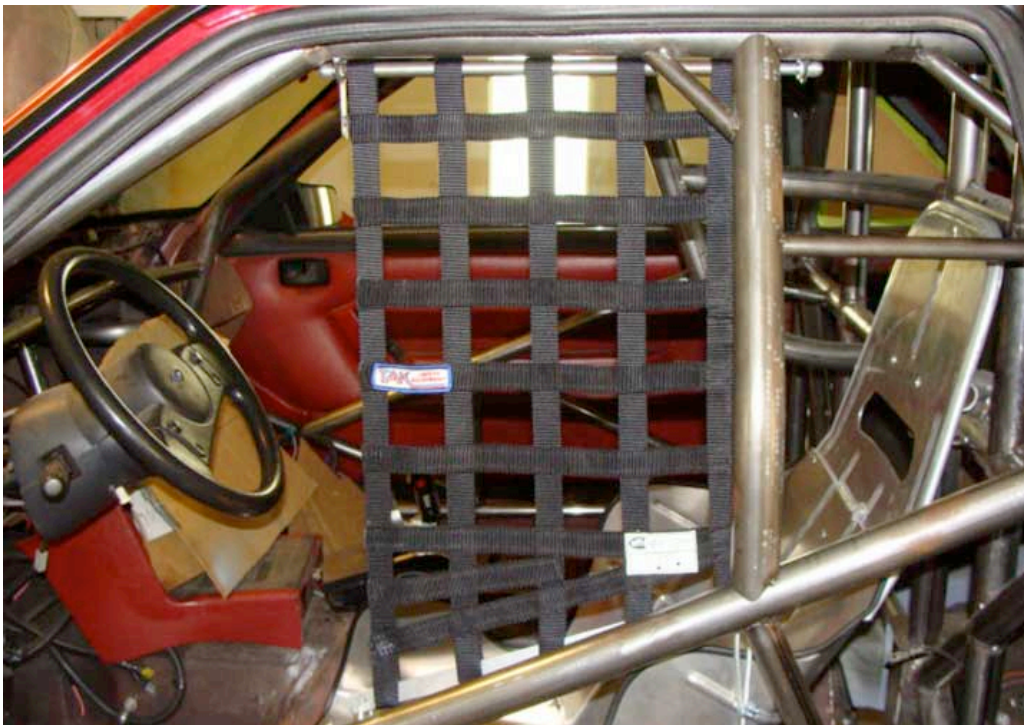
Window net installed
