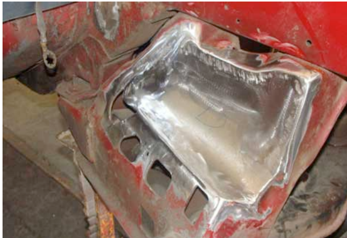
This is the finished product after lots of bending and trimming. Sure would have been easier to just bolt in an aftermarket K-member but NHRA said no.
