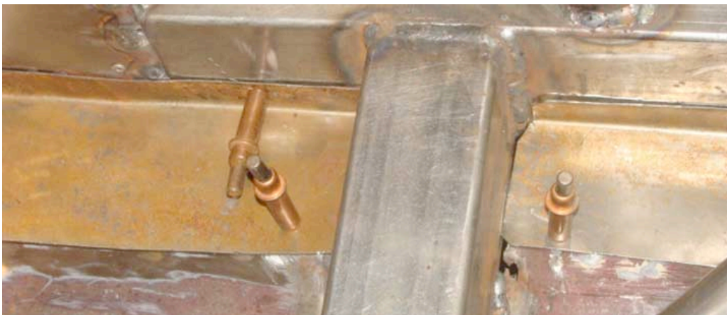
I also made a couple outer pieces between the new frame rails and the rocker panels.
