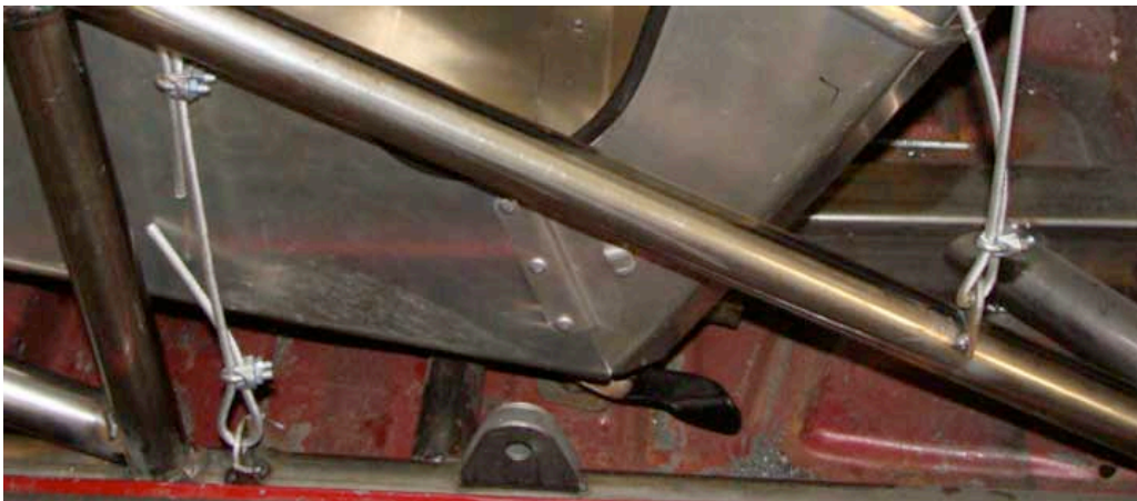
The cables at the bottom are used to attach the net to the rocker sill bar and diagonal. The cables will be trimmed to fit in final assembly.
