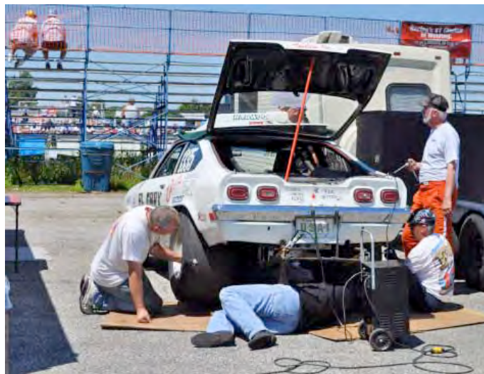
Above, right: The "Al Gary" team also were able to repair the damaged Dana, rebuilding it in the Vega at the track, and they were ready for the race.
